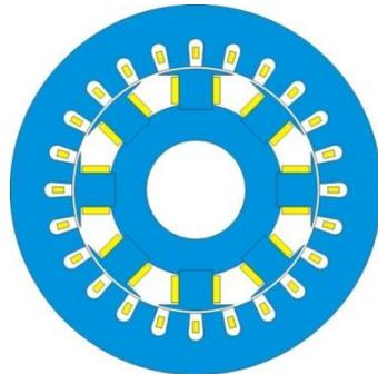
Figure 5: SC motor (rotor sc coil)
