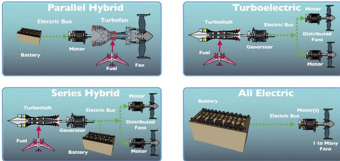
Figure 1: Alternative distributed electrical propulsion configurations (source NASA [3])
