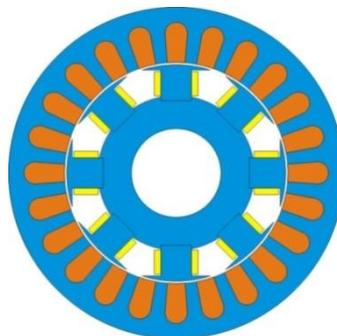
Figure 3: Excited synchronous motor
