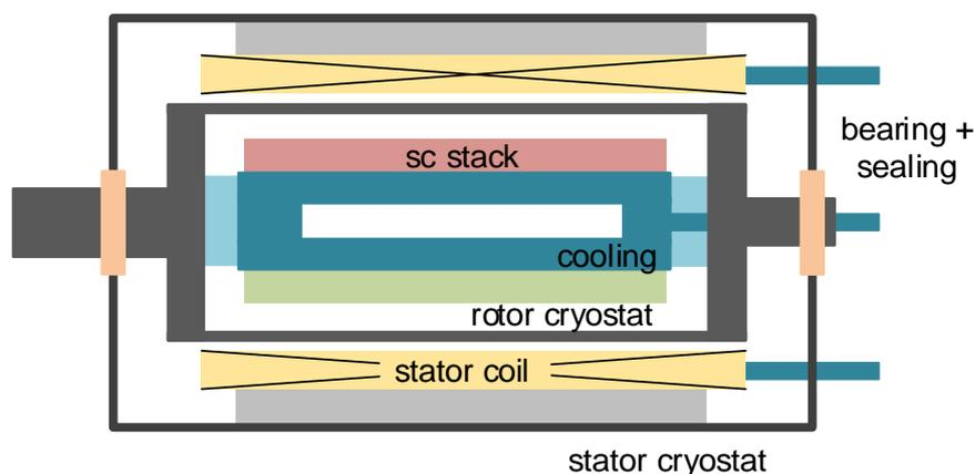
Figure 7: Example of motor cryostat
