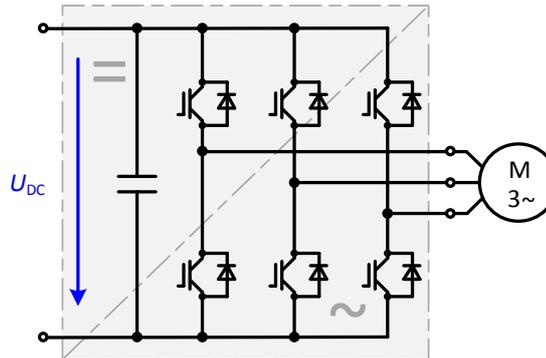
Figure 9: common 3 phase inverter topology
